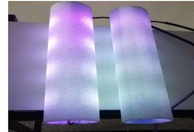
Tiokraft flask for photocatalysis, which uses active hydroxyl radicals ( $\text{OH}$ ) to destroy or damage all organic substances such as viruses, bacteria, fungi etc.
